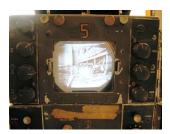
I hooked it all up, and brought the chain up with a vairac. It blew the main fuse at about 75 volts. Now I really had to CHECK the &%#@ caps! I found a bad electrolytic, and just happened to have a new one in stock!!!
